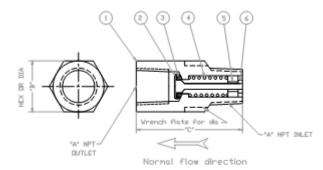
Rvi-05 The flow arrow above is shown as a relief valve, but it can be also used as a check valve when installed in reverse.
