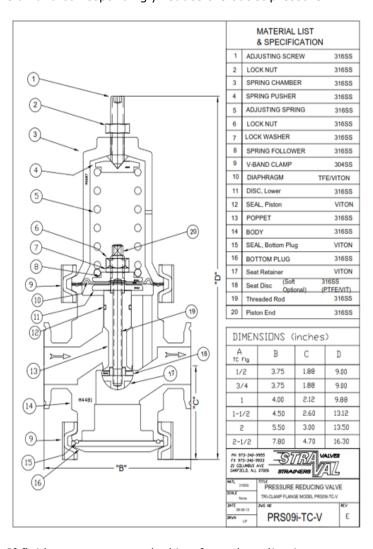
If fluid was or gas was leaking from the adjusting screw, the diaphragm (10) is suspect. Inspect the diaphragm, replace if torn, abraded, or delaminated or otherwise damaged or cut. Sealing area of the diaphragm should be free from tears or cuts, otherwise external leakage will occur. Examine to see if there are signs the diaphragm pulled away from the outer clamped seating area.
